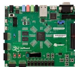
Xilinx ZedBoard Zync-7000 SoC (x1) 2 x USB (UART + JTAG) SERVER Intel Xeon Only for programming & debugging
