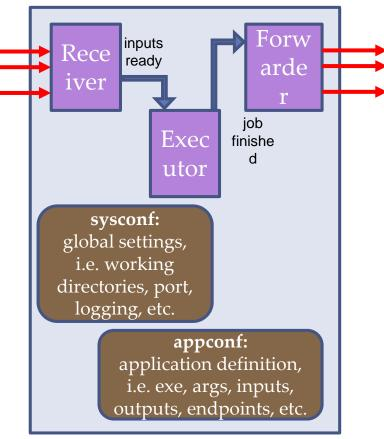
Also requires 2 config files in order to costumize the node according to the workflow definition
